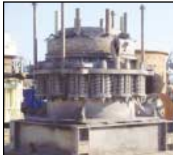
SYMONS-NORDBERG 5-1/2' Shorthead Cone Crusher
