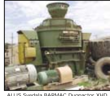
ALLIS Svedala BARMAC Duopactor XHD, Model 9600 MKIII Vertical Shaft Impact Crushers, (2) 300 HP
