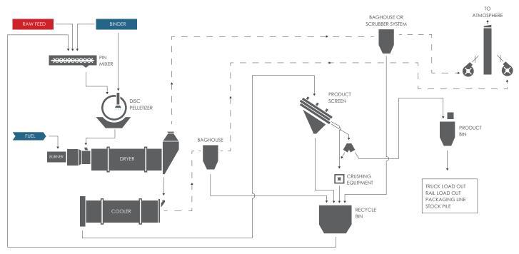
The diagram above illustrates a typical disc pelletizing system with a preconditioning step. The preconditioning step in the mixer helps to make the process more efficient and more effective by pre-mixing the material and binder in a pin mixer or pugmill mixer.
